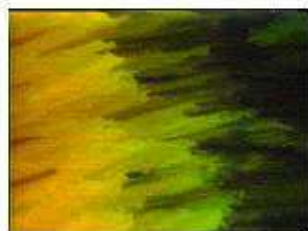
Photo of a smectic phase (using polarizing microscope)
