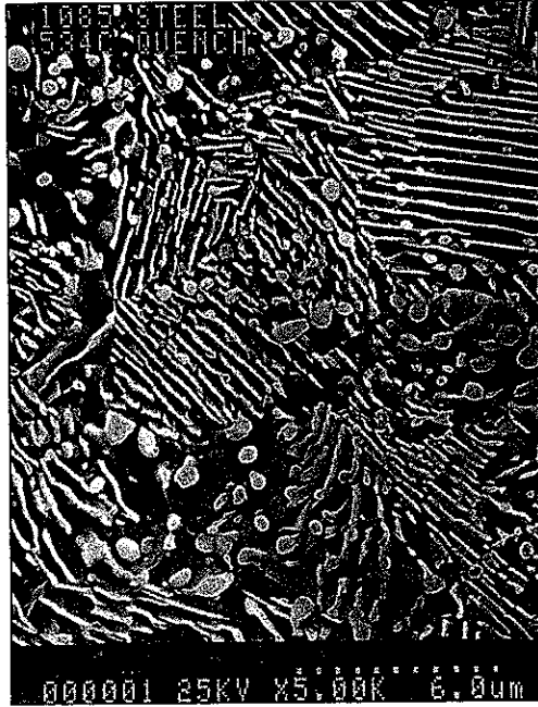
FIGURE 7.8-3 Structure of the eutectoid composition 0.77 wt. % C steel. The eutectoid constituent, called pearlite, has a lamellar (layered) morphology consisting of alternating plates of \alpha Fe (light areas) and \text{Fe}_3\text{C} (dark areas).
